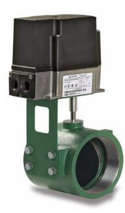
The Eclipse BV-Pak is a fully assembled package that makes ordering simple and installation efficient. It is typically used for the regulation of air or fuel-gas in combustion systems where it serves as the control element in a temperature control loop. It does not provide tight shut-off. The assembly includes an Eclipse catalog 902 Trilogy T500 series actuator mounted to a catalog 720 butterfly valve with bracket, fasteners and coupling.
